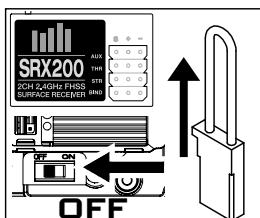
Remove the Bind Plug, then power off the receiver to save the settings.
