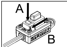
1. Connect a battery. Press and hold the set button and turn on ESC. The RED LED will flash.
