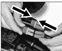
Connect a fully charged battery pack to the ESC.
