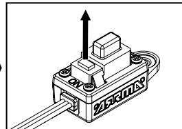
3. To enter the selected variable, release the set button on the desired number of flashes/beeps.
