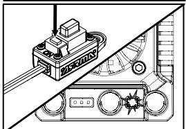
1. Throttle trigger in neutral position - press set button (1 Green flash)
