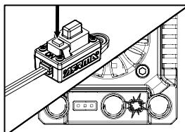
4. Using the tuning chart, press the 'set' button until the number of red LED flashes and short beeps equals the required value.
